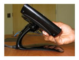
Pull the latch toward the touchpanel to lock onto dock. Ensure the touchpanel is securly locked on docking station
